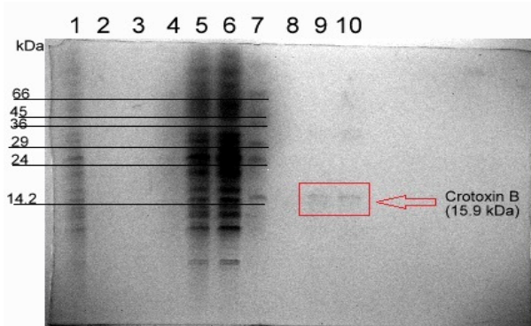
Figure 6. SDS-PAGE gel analysis of samples taken from cell cultures incubated using the optimal conditions (37°C, 0.5 mM IPTG concentration) and the affinity chromatography purification of the recombinant protein using Tris-HCl buffer (pH=7.6). (1) – 120 min after induction; (2) – 60 min after induction; (3) – before induction; (4) - Molecular Weight Marker 14-66 kDa (Sigma-Aldrich), (5) – elution fraction 1, (6) – elution fraction 2, (7) – elution fraction 3.
