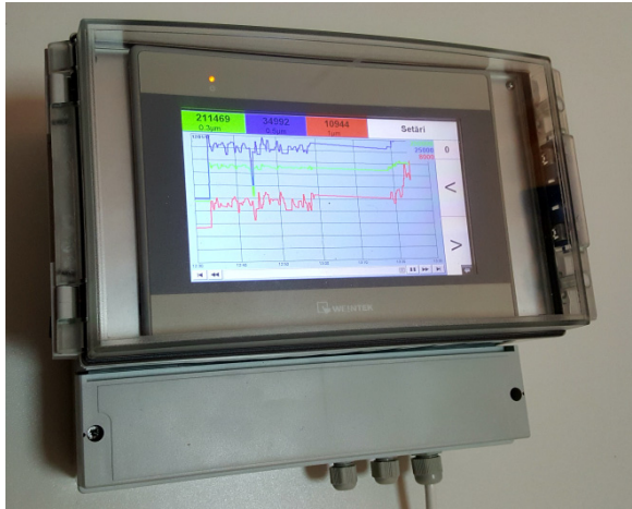
Figure 1. DUMO System for monitoring submicron airborne dust particles (Manufacturer SC ELECTRONIC APRIL, Aparatura Electronica Speciala SRL, Cluj-Napoca, Romania)
