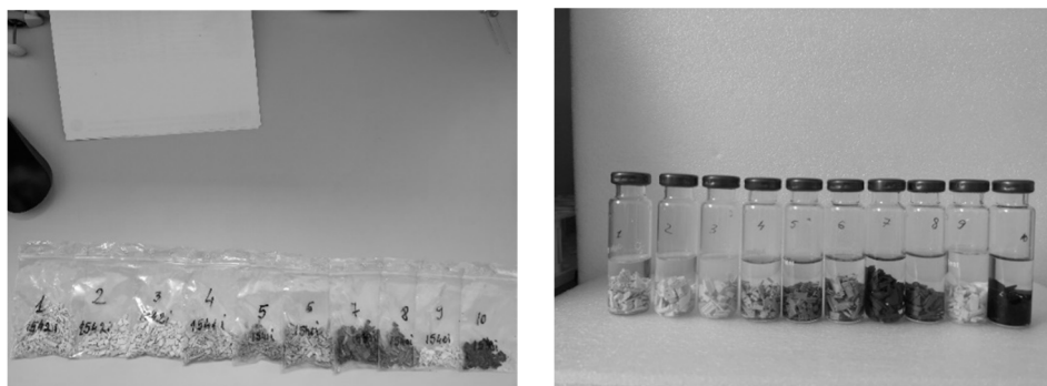
Figure 2. Chopped plastic materials (left) and Headspace extraction of volatile compounds from plastics (right)
