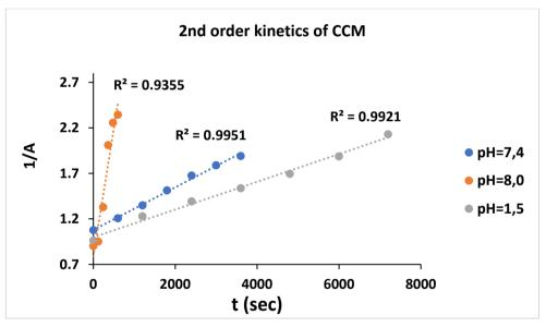
Figure 12 B. The second order degradation plot of CCM at different pH values and at 37°C.
