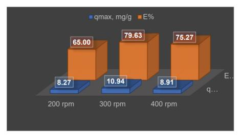
**Figure 5.** The maximum efficiency and adsorption capacity for Zn<sup>2+</sup> biosorption process onto RGP biomass; the influence of stirring rate.
