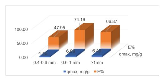
**Figure 6.** The effect of grain size biosorbent over the amount of  $Zn^{2+}$  uptake onto RGP biosorption (224 mg  $Zn^{2+}/L$ , 300 rpm, grain size biomass granulation 0.4-0.6, 0.6-1 mm, >1 mm, 2 g RGP/ 100 mL).
