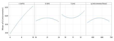
Figure 3. Factorial plot for the diameter vs. the parameters (c, U, I, q)
