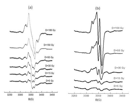
**Figure 2.** EPR spectra of γ-irradiated: (a) steviol and (b) sucrose, at different absorbed doses.
