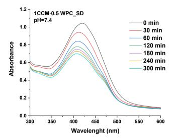
Figure 11.A. The UV-vis spectra of the decrease in time of CCM absorbance in 1CCM-0.5WPC\_SD at pH 7.4
