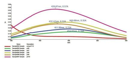
Figure 1. UV-Vis spectra of AgNPs obtained at different pH values
