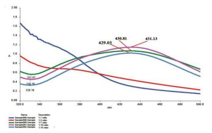
Figure 3. UV-Vis spectra of AgNPs obtained at different fruit extract: AgNO<sub>3</sub> ratios
