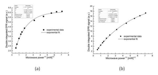
Figure 4. EPR power saturation curves for of irradiated steviol (a) and sucrose (b)
