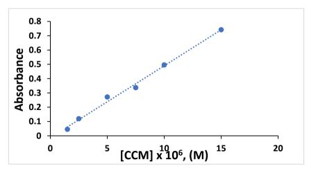
**Figure 10.** Calibration curve of CCM in ethanol. Characteristics of regression line are: y = 50361x - 0.0137, where x is curcumin concentration, and R<sup>2</sup> = 0.9932.
