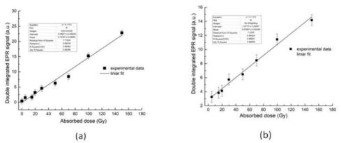
**Figure 3.** Dose response relationship for (a) steviol and (b) sucrose as a function of the irradiated dose (errors bars are provided with 6% error limits).
