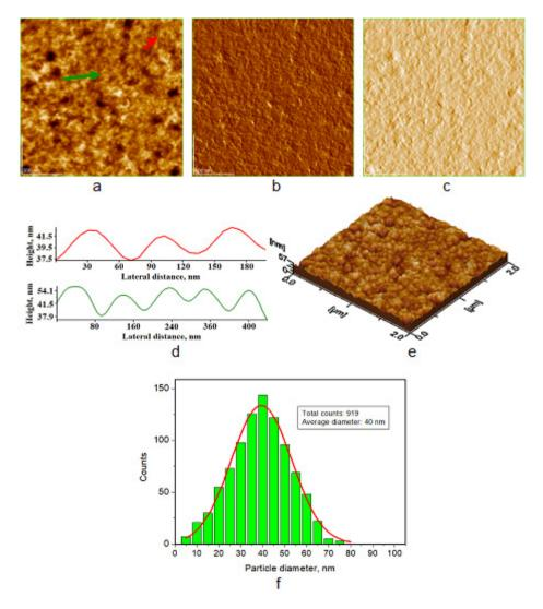
**Figure 3.** AFM images of the CCM-WPC complex, obtained at pH 7.4, adsorbed on glass and naturally dried: a) topographic image, b) phase image, c) amplitude image, d) profile along the arrow in panel (a), e) tridimensional image and f) histogram of particle size distribution. Scanned area 2 μm x 2 μm.
