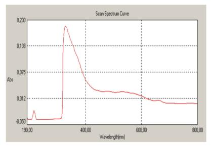
Figure 3. UV-VIS spectrum of the red grape extract (extraction in EtOH, 20°C (293K), dilution 1:100).
