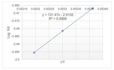
Figure 8. Plot of lnKd versus 1/T for  $Zn^{2+}$  biosorption onto RGP (Ci = 272 mg  $Zn^{2+}/L$ , 2 g RGP, 0.6 < d < 1.0 mm, 300 rpm).
