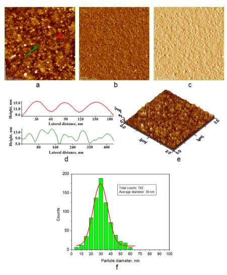
**Figure 1.** AFM images of CCM NPs adsorbed on glass and naturally dried: a) topographic image, b) phase image, c) amplitude image, d) profiles along the arrows in panel (a), e) tridimensional image and f) histogram of particle size distribution. Scanned area 2 μm x 2 μm.
