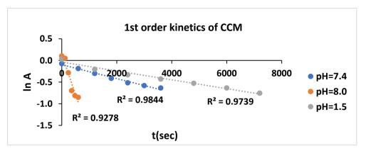
Figure 12 A. The first order degradation plot of CCM at different pH values and at 37°C.
