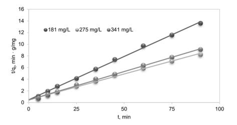
Figure 9. Plots of the pseudo-second-order kinetic model of Zn<sup>2+</sup> biosorption, onto RGP biomass.
