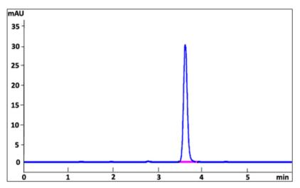
Figure 2. Typical chromatogram for IND assay from a TTS sample
