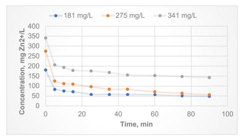
Figure 4. The influence of the initial Zn<sup>2+</sup> concentration over the time evolution for biosorption onto RGP (181–341 mg Zn<sup>2+</sup>/L, 2 g RGP, 0.6-1.0 mm, 293 K, pH= 6.3, 200 rpm).
