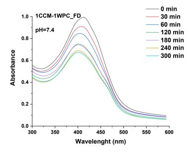
**Figure 11.B.** The UV-vis spectrum of the decrease in time of CCM absorbance in 1CCM-1WPC FD complex at pH 7.4
