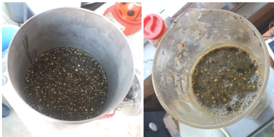
Figure 5. The anaerobic co-digestion suspension consisted of animal slurry, wastewater and corn grain mixture
