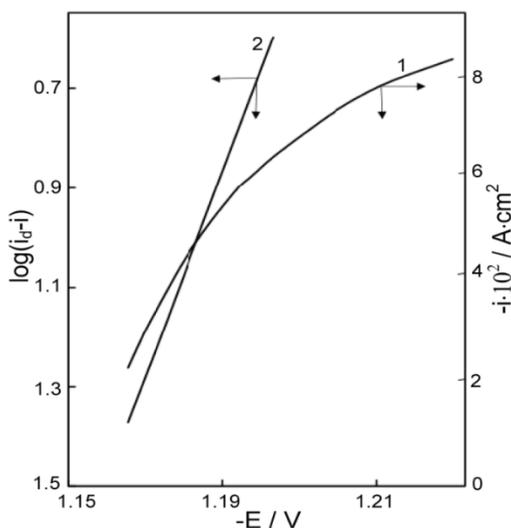
**Figure 5.** Cathodic polarization of tungsten electrode (1) and its analysis in the semi-logarithmic coordinate system (2);  $v = 0.02$  V/s,  $T = 1173$  K,  $C(B_2O_3) = 6 \cdot 10^{-4}$  mol/cm<sup>3</sup>.
