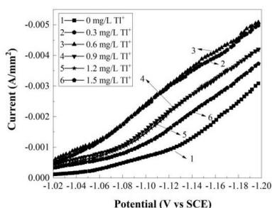
**Figure 6.** Cathodic polarization curves measured in electrolytes with different thallium( I ) ion concentrations at a scan rate of 10 mV s<sup>-1</sup>. Electrolyte: 35.46 g/L Zn<sup>2+</sup> and 146.05 g/L H<sub>2</sub>SO<sub>4</sub> electrolyte with varied Tl( I ) ions concentration (mg L<sup>-1</sup>); temperature: 38 ± 1 °C.
