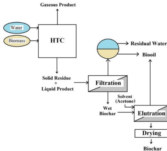
**Figure 9.** Schematic diagram for hydrothermal carbonization process.
