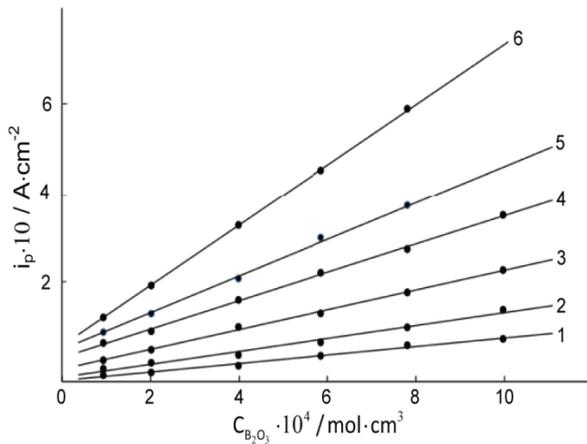
**Figure 3.** Dependence of the peak current on the  $\text{B}_2\text{O}_3$  concentration at different polarization speeds: (1) –  $0.02 \text{ V/s}$ ; (2) –  $0.05 \text{ V/s}$ ; (3) –  $0.1 \text{ V/s}$ ; (4) –  $0.5 \text{ V/s}$ ; (5) –  $1.0 \text{ V/s}$ ; (6) –  $2.0 \text{ V/s}$ ;  $T = 1173 \text{ K}$ .
