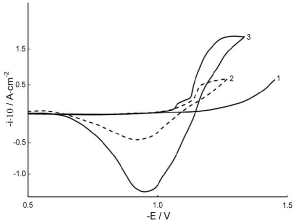
**Figure 2.** Voltammetric dependences of  $\text{Na}_2\text{WO}_4$  melt (1) when added sequentially  $\text{B}_2\text{O}_3$ : (2) –  $1 \cdot 10^{-4} \text{ mol/cm}^3$ ; (3) –  $8 \cdot 10^{-4} \text{ mol/cm}^3$ ;  $T = 1173 \text{ K}$ , cathode – Pt,  $v = 0.1 \text{ V/s}$ .
