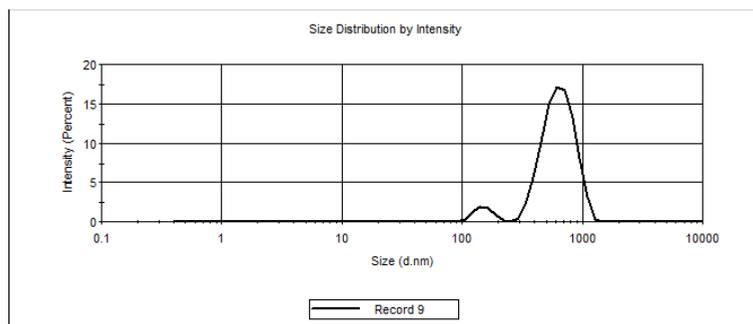
**Figure 5.** DLS distribution of particle sizes of Tuf 2
