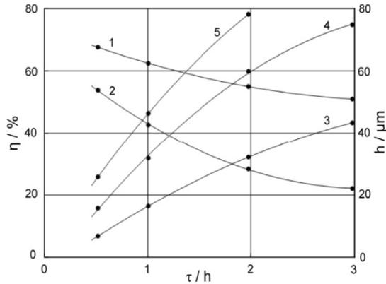
**Figure 7.** The dependence of the thickness of the tungsten coating (1-3) and the yield of tungsten according to the current (4) and (5) on steel samples from the duration of electrolysis at the current density: (1) and (4) – 4 A/dm<sup>2</sup>; (2) and (5) – 6 A/dm<sup>2</sup>; (3) – 8 A/dm<sup>2</sup>; T = 1173 K.
