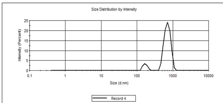
**Figure 4.** DLS distribution of particle sizes of Tuf 1
