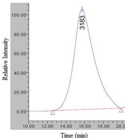
**Figure 1:** Chromatogram of polymycene-block-polystyrene copolymer (Table 1, Entry 4)
