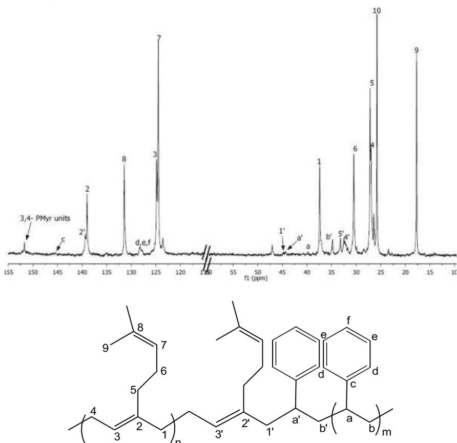
**Figure 3:** <sup>13</sup>C NMR (75 MHz, CDCl<sub>3</sub>) spectrum of myrcene-styrene copolymer (Table 1, Entry 4) and assignments.
