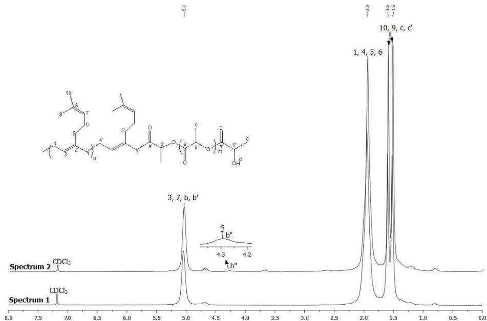
**Figure 6:** Spectrum 1: <sup>1</sup>H NMR (300 MHz, CDCl<sub>3</sub>) spectrum of homopolymyrcene; Spectrum 2: <sup>1</sup>H NMR (300 MHz, CDCl<sub>3</sub>) spectrum of myrcene-lactide copolymer (Table 2, Entry 4)
