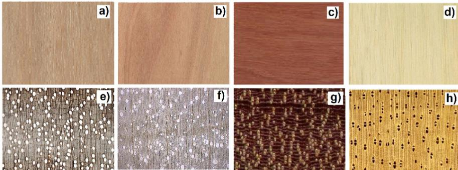
**Figure 1.** Wood Macroscopic Tangential Section (Polished) a) CE b) EG c) WT d) NC, Wood Microscopic Transverse Section - e) CE f) EG g) WT h) NC (Adopted from Richter, H.G., Gembruch, K., and Koch, G. 2014 onwards. CITESwoodID: descriptions, illustrations, identification, and information retrieval. In English, French, German, and Spanish. Version: 17th February 2019. delta-intkey.com)
