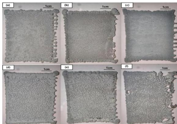
**Figure 2.** Photographs of zinc deposits showing the effect of various electrolyte thallium( I ) ion concentrations. (a) 0.0 mg L<sup>-1</sup>, (b) 0.3 mg L<sup>-1</sup>, (c) 0.6 mg L<sup>-1</sup>, (d) 0.9 mg L<sup>-1</sup>, (e) 1.2 mg L<sup>-1</sup>, (f) 1.5 mg L<sup>-1</sup>.
