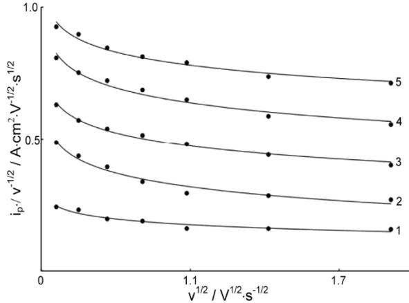
**Figure 4.** Dependence  $i_p/v^{1/2} - v^{1/2}$  for the tungsten-containing ions electroreduction process at  $C(B_2O_3) \cdot 10^4 \text{ mol/cm}^3$ : (1) – 2 mol/cm<sup>3</sup>; (2) – 6 mol/cm<sup>3</sup>; (3) – 8 mol/cm<sup>3</sup>; (4) – 10 mol/cm<sup>3</sup>; (5) – 12 mol/cm<sup>3</sup>; T = 1173 K.
