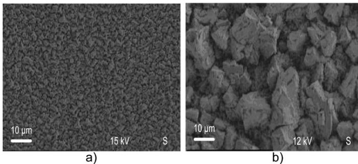
**Figure 8.** SEM image of tungsten coating deposited on steel substrate: a) 20 s; 8 A/dm<sup>2</sup>; b) 60 s, 15 A/dm<sup>2</sup>.
