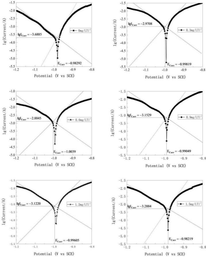
**Figure 7.** Corrosion potential and corrosion current density obtained by the slope extrapolation method at a scan rate of 10 mV s<sup>-1</sup>. Electrolyte: 35.46 g/L Zn<sup>2+</sup> and 146.05 g/L H<sub>2</sub>SO<sub>4</sub> electrolyte with varied TI<sup>+</sup> (I<sup>-</sup>) ions concentration (mg L<sup>-1</sup>); temperature: 38 ± 1 °C.
