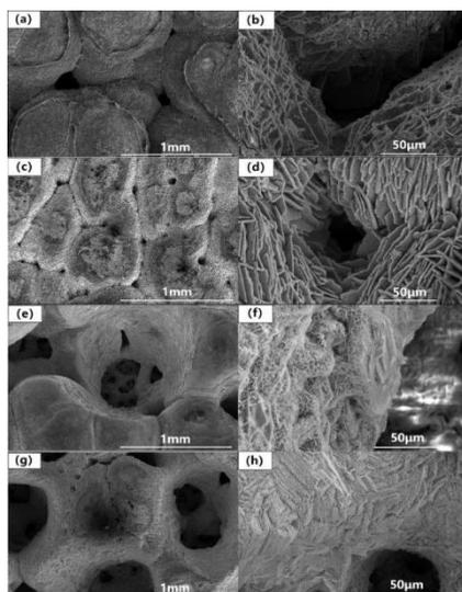
**Figure 3.** SEM micrographs showing the effect of electrolyte thallium( I ) ion concentrations on the morphology of deposits after electrowinning at 518.86 A m<sup>-2</sup> for 24 h. (a) (b) 0.0 mg L<sup>-1</sup>, (c) (d) 0.6 mg L<sup>-1</sup>, (e) (f) 0.9 mg L<sup>-1</sup>, (g) (h) 1.5 mg L<sup>-1</sup> at different magnifications.
