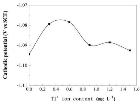
**Figure 5.** Effect of thallium( I ) ion concentration on cathodic potential curves for zinc deposition at a cathodic current density of  $518.86 \text{ A m}^{-2}$ . Electrolyte:  $35.46 \text{ g/L Zn}^{2+}$  and  $146.05 \text{ g/L H}_2\text{SO}_4$  electrolyte with varied  $\text{Tl(I)}$  ions concentration ( $\text{mg L}^{-1}$ ); temperature:  $38 \pm 1 \text{ }^\circ\text{C}$ .
