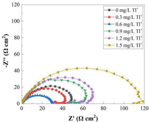
**Figure 9.** Nyquist plots measured in electrolytes with different thallium( I ) ion concentrations at a voltage of -1.05 V. Electrolyte: 35.46 g/L Zn<sup>2+</sup> and 146.05 g/L H<sub>2</sub>SO<sub>4</sub> electrolyte with varied Tl( I ) ion concentration; temperature: 38 ± 1 °C.
