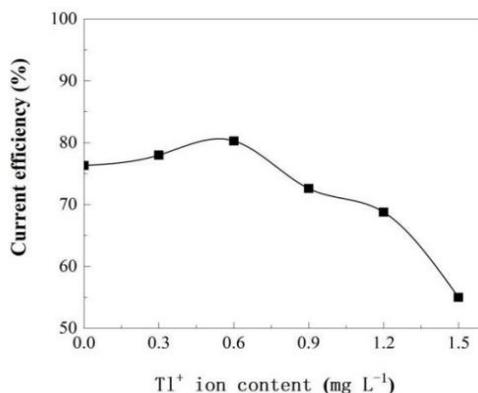
**Figure 1.** Effect of thallium( I ) ion content on the current efficiency of 24 h zinc deposition at a cathode current density of  $518.86 \text{ A m}^{-2}$ . Electrolyte:  $35.46 \text{ g/L Zn}^{2+}$  and  $146.05 \text{ g/L H}_2\text{SO}_4$  electrolyte with varied Tl( I ) ions concentration ( $\text{mg L}^{-1}$ ); temperature:  $38 \pm 1 \text{ }^\circ\text{C}$ .
