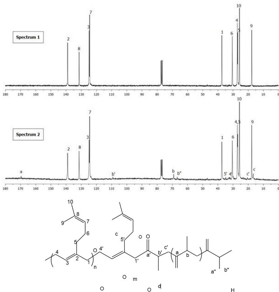
**Figure 7:** Spectrum 1:  $^{13}\text{C}$  NMR (75 MHz,  $\text{CDCl}_3$ ) spectrum of homopolymyrcene; Spectrum 2:  $^{13}\text{C}$  NMR (75 MHz,  $\text{CDCl}_3$ ) spectrum of myrcene-lactide copolymer (Table 2, Entry 4) and assignments
