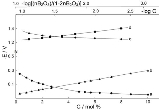
**Figure 1.** Dependence of potentials of platinum-oxygen (a) and tungsten (c); electrodes on  $B_2O_3$  concentration and their analysis in the logarithmic coordinate system: (b) – platinum-oxygen electrode; (d) – tungsten electrode. ( $T = 1173$  K).
