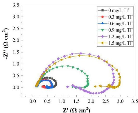
**Figure 10.** Nyquist plots measured in electrolytes with different thallium( I ) ion concentrations at a voltage of -1.1 V. Electrolyte: 35.46 g/L  $Zn^{2+}$  and 146.05 g/L  $H_2SO_4$  electrolyte with varied  $Tl(I)$  ion concentration; temperature:  $38 \pm 1$  °C.
