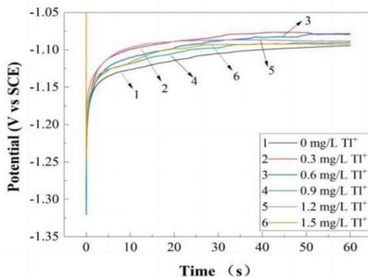
**Figure 4.** Chronopotentiometric curves measured in electrolytes with different thallium( I ) ion concentrations at  $518.86 \text{ A m}^{-2}$  cathode current density. Electrolyte:  $35.46 \text{ g/L Zn}^{2+}$  and  $146.05 \text{ g/L H}_2\text{SO}_4$  electrolyte with varied  $\text{Tl(I)}$  ions concentration ( $\text{mg L}^{-1}$ ); temperature:  $38 \pm 1 \text{ }^\circ\text{C}$ .
