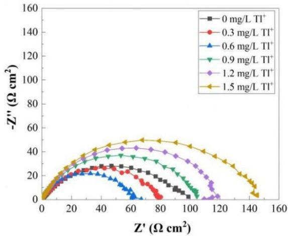
**Figure 8.** Nyquist plots measured in electrolytes with different thallium( I ) ion concentrations at a voltage of -1 V. Electrolyte: 35.46 g/L Zn<sup>2+</sup> and 146.05 g/L H<sub>2</sub>SO<sub>4</sub> electrolyte with varied Tl( I ) ion concentration; temperature: 38 ± 1 °C.
