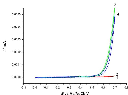
**Fig. 4.** The voltammograms of PIGE modified electrodes in contact with  $1\text{ M KOH} + 1\text{ M CH}_3\text{OH}$ . 1-blank electrode; 2- $\text{YFeO}_3$ ; 3- $\text{YCo}_{0.5}\text{Fe}_{0.5}\text{O}_3$  and 4- $\text{YCoO}_3$ .
