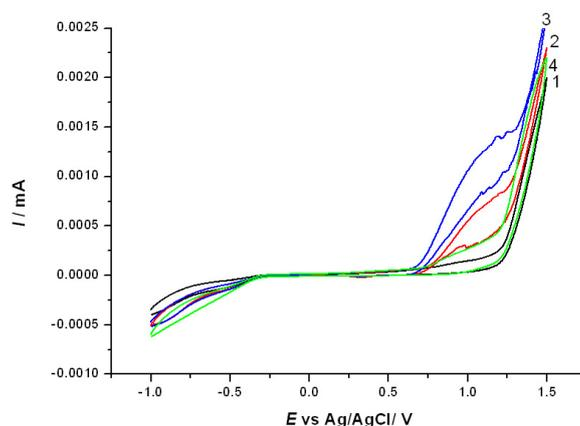
**Fig. 2.** The voltammograms of modified electrodes in contact with 0.1 M solution of KOH. 1- blanc electrode; 2 -  $\text{YFeO}_3$ ; 3 -  $\text{YFe}_{0.5}\text{Co}_{0.5}\text{O}_3$  and 4 -  $\text{YCoO}_3$ .
