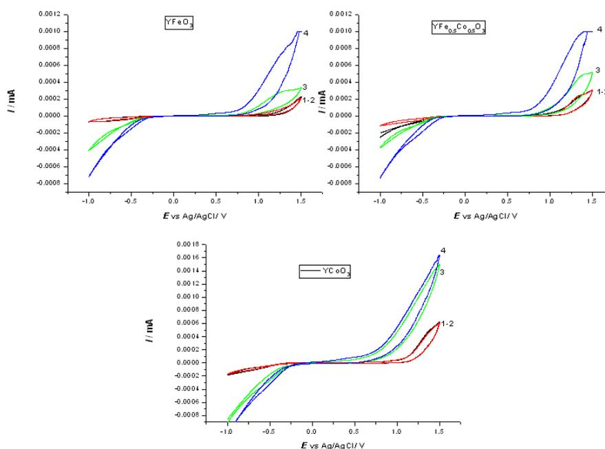
**Fig. 4.** The investigated compounds in: 1-phosphate buffer solution; 2-phosphate buffer +  $10^{-3}$  M  $\text{H}_2\text{O}_2$ ; 3-phosphate buffer +  $10^{-2}$  M  $\text{H}_2\text{O}_2$ ; 4-phosphate buffer +  $10^{-1}$  M  $\text{H}_2\text{O}_2$ .
