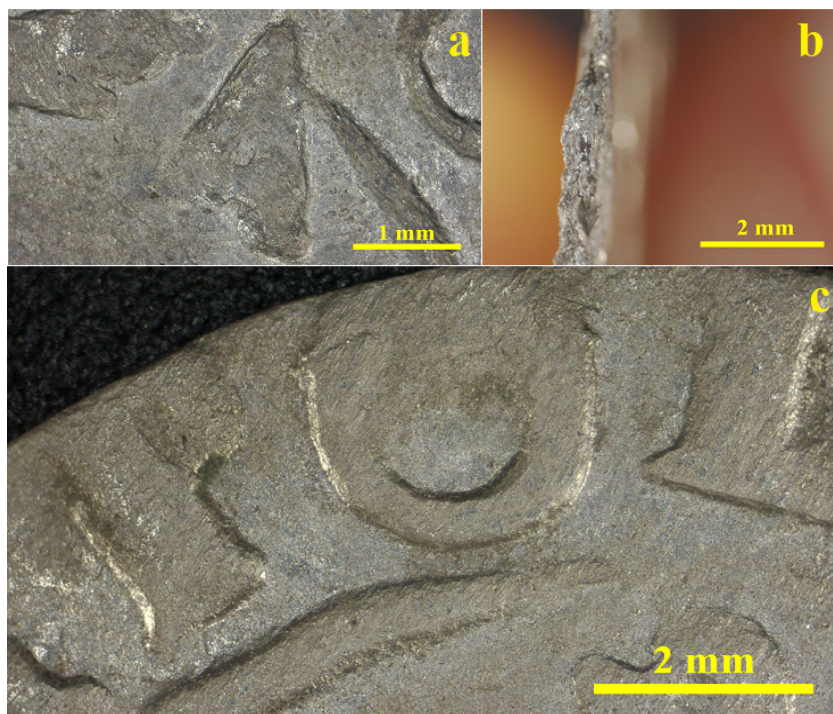
Figure 3. Macrostructural details observed at low magnification (x10) in reflected light of the abnormally corroded poltorak from 1624: a) detail on year distinctive number 4, b) coin's edge aspect and c) aspect of the coin's text.
