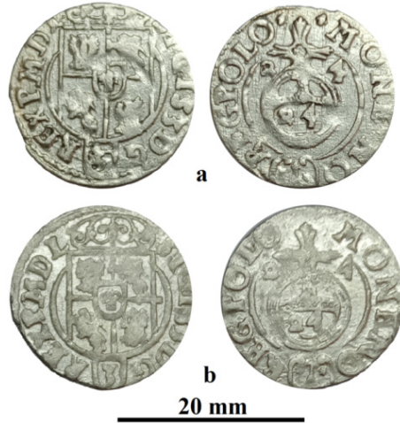
Figure 1. Investigated samples: a) well preserved póltorak issued in 1624 and b) abnormally corroded póltorak from 1624.
